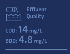
The effluent quality levels are on average at least 93% better than the local normative (COD: 200 mg/L BOD: 100 mg/L).
